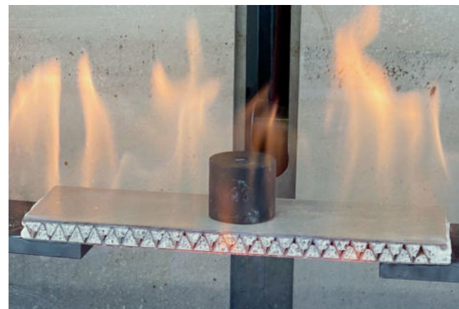
FireAway sandwich testing: No degradation after 2 hours in 950°C gas flame.
